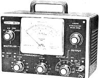
Heathkit AG-9U audio signal generator Heathkit AG-9U audio signal generator **AO-1U.** Inexpensive audio generator covering 20 c/s-150 Kc/s sine wave, 20 c/s-25 Kc/s square wave. Output up to 10V RMS sine wave or 80V peak-to-peak square wave. Size:  $9\frac{1}{2} \times 6\frac{1}{2} \times 5$  in. Price (kit): £14 15s.; (assembled): £21 5s.
