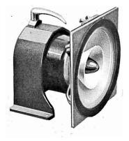
**Trebax 5K/20XL.** Horn loaded pressure tweeter. Built in L/C crossover (5,000 c/s) and attenuator. Suitable for inclusion in systems of up to 20W. Dispersion angle 90]. Price: £7 13s. 9d.
