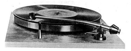
**"600".** Variable reluctance turnover cartridge.  $\frac{1}{2}$  in. centre, mounting holes. Diamond stylus for LP, sapphire for 78. Output voltage  $3\cdot 2$  mV. Range 20 c/s-21 Kc/s  $\pm 2$  dB. P.w. 5 gm. Load impedance 68K. Price: £8 8s. (U.K. purchase tax £1 7s. 4d.).
