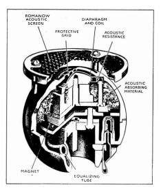
**Fig 11** Sectional view of an STC moving-coil microphone, showing the internal construction. Note the equalising tube.
