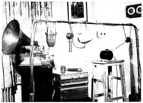
Fig 4. A series of microphones showing the work of BBC research engineers in the 25 years up to 1949. L to R, BBC-Marconi ribbon; moving coil on hand grip; condenser in "bomb" mounting; Reisz carbon; Round-Sykes "Magnetophone" (on stool); Peel-Connor Carbon with trumpet: BBC-Marconi lip microphone (on box). The gramophone was used to replay the voice of Dame Nellie Melba in a broadcast recalling the past.
