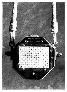
cavity, in which were located the two carbon electrodes and the finely divided carbon granules, retained by a thin, non-metallic diaphragm. The diaphragm was of mica in the early models but impregnated paper was later substituted to overcome the pronounced resonance of the mica at about 4,500 Hz. The axial frequency response of the modified microphone was sensibly flat up to about 500 Hz, above which it rose fairly sharply and at 8,000 Hz was about 10 dB up.
