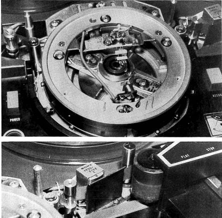
Fig 4. The helical-scanning system used in the Sony home video tape machine. This is fully explained in the text.
