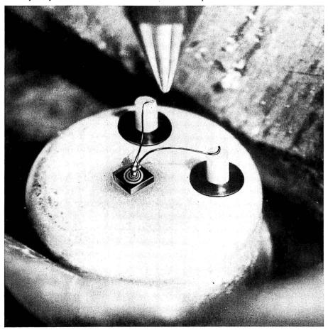
Fig 8. Fixing the base wire to a Mullard transistor.
