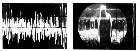
Fig 1. Waveform of sound (a) compared with waveform of television line (b). The period of the latter is only about 64 microseconds, and component frequencies within this rise to some 5MHz.
