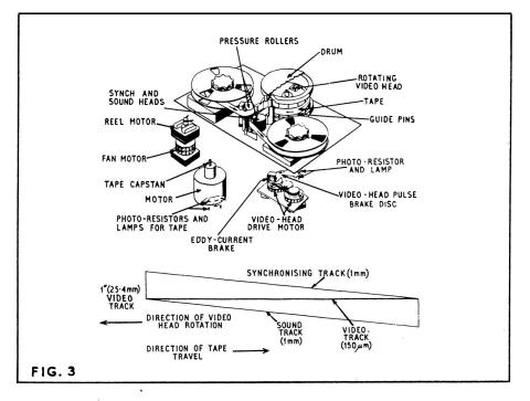
Fig 3. The semi-professional helical-scanning system.
