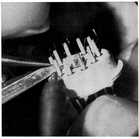
Fig 5. Fixing an integrated circuit to its mounting. Mullard Ltd.
