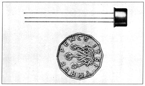
Fig 6. General purpose junction transistor by Mullard Ltd.
