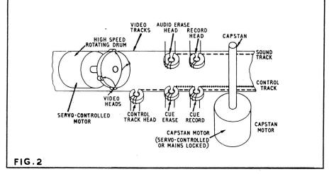
Fig 2. The transverse scanning system used in professional video tape machines.
