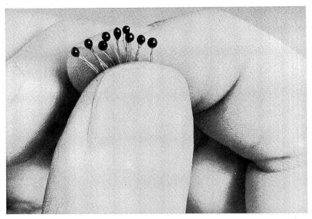
Fig 7. Collection of microminiature silicon planar epitaxial transistors by Mullard Ltd.
