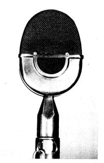
Fig 5. BBC-Marconi ribbon microphone.
