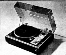
Model SR4040. Two-speed Manual Turntable. Complete with magnetic cartridge. 4pole synchronous capacitor start motor. Wow and flutter less than o-o.8%.
