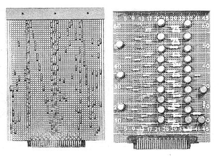
produce board on 0·1-inch pitch, which involved the development of new tooling, but owing to the nature of the problems concerned with this smaller pitch—the copper strips had to be no more than 0·075 inch wide and the centres pierced accurately with holes of the largest practical diameter, which worked out to be 0·04 inch. This tooling development extended over some eighteen months.
