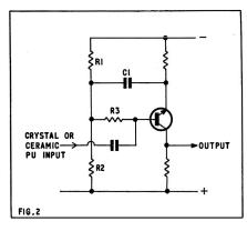
**Fig 2.** The ceramic/crystal cartridge input circuit of the Tripletone 8+8.
