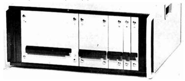
Fig 16. Vero Module Rack Unit fitted in an Alton Case.
