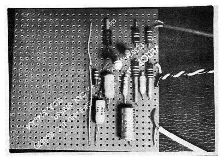
Fig 8. A simple tape head amplifier on Veroboard.
