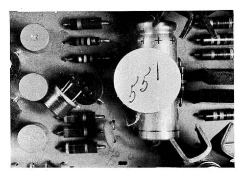
**Fig 5.** Close-up of plug-in transistor (a) and group of plug-in transistors (b) in the Fisher 200-T tuner-amplifier.
