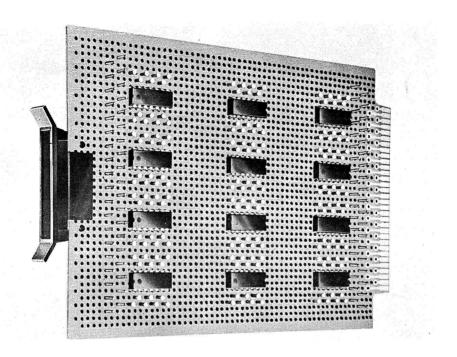
$\label{eq:FigS} \textbf{Finger Board with i.c's. mounted, showing one style of Vero Handle.}$
