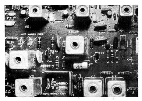
"modules") are used for each main section and sub-section. One notable exception, however, is the *Sansui* 250 tuner-amplifier, already referred to, in which a wired circuit is adopted exclusively (**Fig 9**).
