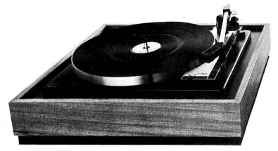
The HT 70 is a luxury single player with a fully counterbalanced pickup arm, deep rim  $4\frac{1}{2}$  lb die cast turntable, rotating record stub spindle, viscous damped cueing device, slide-in cartridge holder, anti-skate control, and a 4 pole dynamically balanced synchronous motor.
