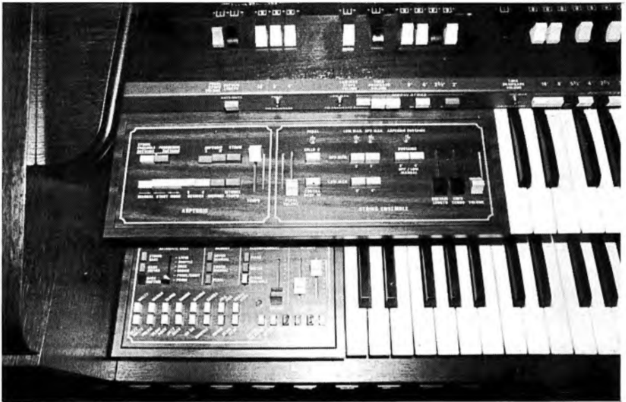
The left hand cheek blocks of the Eminent 2000 showing the Arpeggio, String Ensemble and Rhythm unit controls. The rhythm unit contains the controls for the automatic bass, accompaniment and memory.
