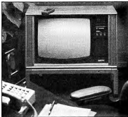
Looking like almost any other CTV the Pye CT494 has both teletext and Prestel facilities using the keypad on top of the set and an infra-red remote control link
