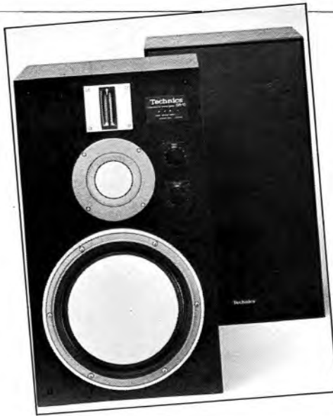
In the Technics SB-10 speaker the bass driver unit at the bottom has a flat diaphragm of honeycomb construction in place of the conventional cone
