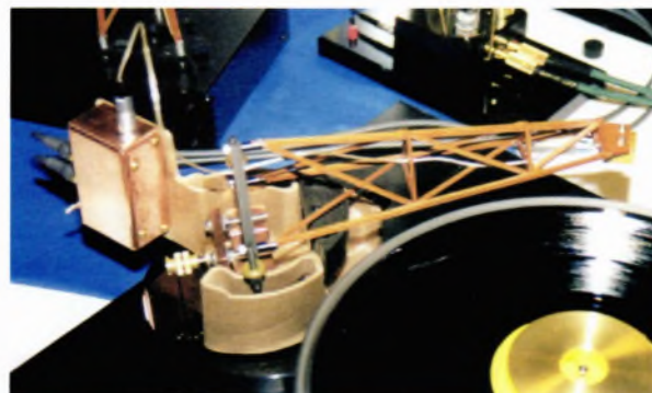
The Golden Gate tonearm, complete with dual damping troughs and rear mounted phono stage.
