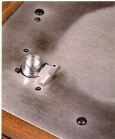
Detail of motor-fixing and top-plate suspension bolts showing black hard-ware associated with Nirvana upgrade.
