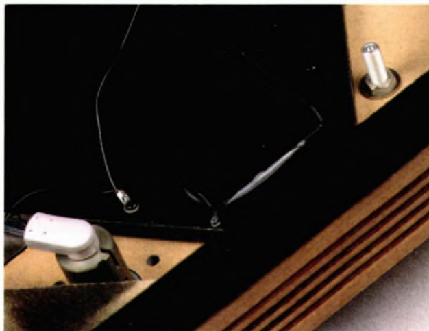
Underside of sub-chassis showing later glued construction.
