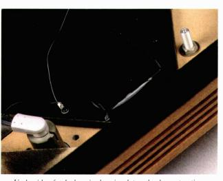
Underside of sub-chassis showing later glued construction.
