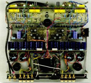
a hybrid amplifier, with a bi-polar input stage and J-fet phase splitters used to feed a hybrid J-fet/12AU7 cascode driver for each channel. The push-pull EL34s run in Class AB and the entire circuit is dual mono down to separate windings on the
