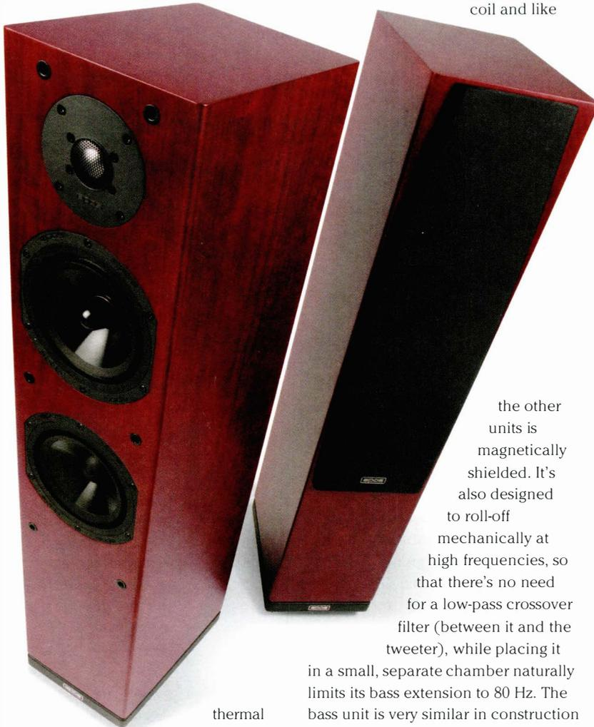
thermal compression, improving sound quality considerably. The tweeter crossover is centred on 5 kHz, which is significantly higher than most other three-way speakers, moving the crossover point away from the area where the ear is most sensitive (circa 2 kHz) as well as spreading the load more evenly between drivers than designs that use the tweeter to lower frequencies.
