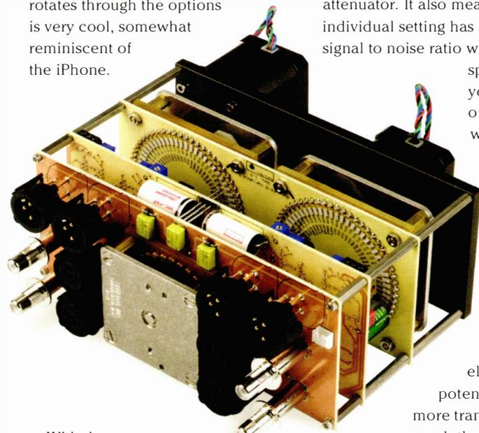
With the base-plate removed it's impossible to miss the array of four, large diameter Shallco switches employed to control level in the four phases of the fully balanced circuit. From which you might deduce that Ayre have simply re-engineered the arrangement used in the K-1xe – but you'd be
