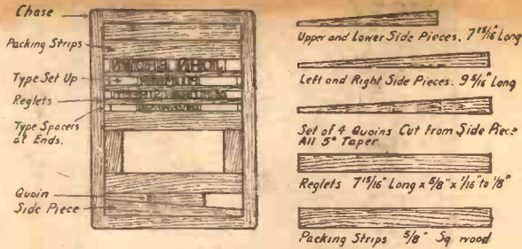
Fig. 4.—How the type is set in the forme.
