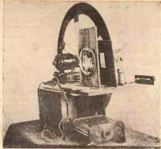
The simple Televisor described in this article.
