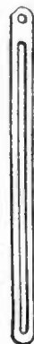
Fig. 10.— The lid stay is made of brass and slotted as shown here.
