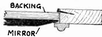
Fig. 5.—A section to show how the mirror is fixed in. Notice the backing held by a "spring" or nail.
