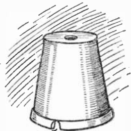
Fig. 3.—How the flower-pot is drilled HOLE TO TAKE GLASS TUBE.
