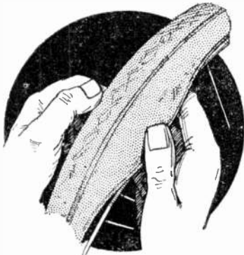
When you suspect a puncture, carefully go over the cover first, when you may be able to locate the cause.
