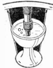
A simple test to find whether the valve is leaking. If there is a leak, air bubbles will rise.
