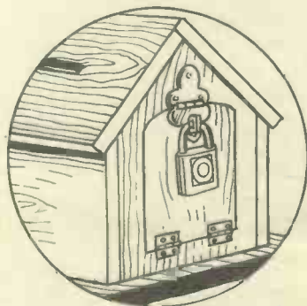
Fig. 4—A detail of how the door is hinged and locked.
