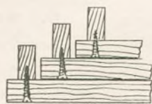
Fig. 4—A section showing how they fit into each other.
