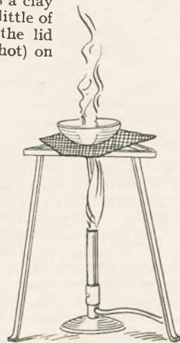
The evaporating process for obtaining hypo.
