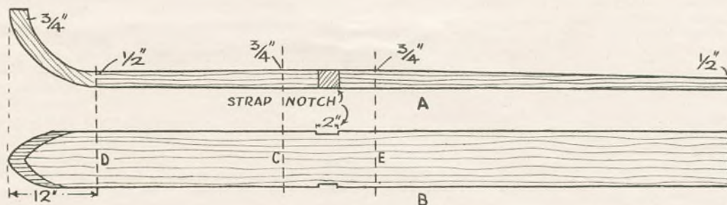
Fig. 1—A side and top view of the ski showing shape and dimensions.
