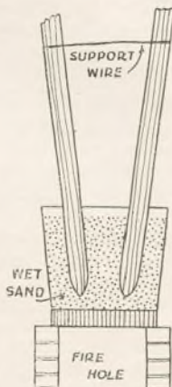
Fig. 3—How the band is steamed (in section).
