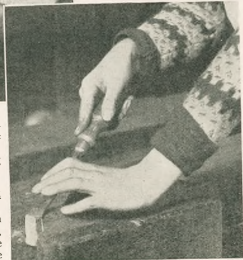
At the top is the chisel held upright for a vertical cut, below it is paring an oblique cut across the work.
