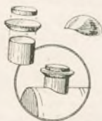
Fig. 3—How the funnel and steam chest are made and fitted.
