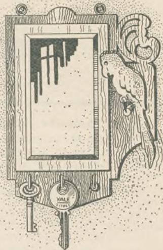
glue the overlay evenly over the glass aperture to show a  $\frac{1}{16}$ in. flange all round. If the back is cut from plywood, the waist—which should be cut out in one piece—can be reduced to suit the thickness of the glass by removing a ply. On the other hand, you could "pack" the mirror at the back with rectangles of cardboard until level with the work.
