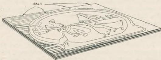
*Four pieces of wood nailed together with pattern pasted on selected.* A coarse saw, you will understand, will make a very wide cut between the actual parts and so prevent them coming as close together as they should. Get a fine saw in your machine or handframe, therefore, and if you break any keep to the same grade right through.
