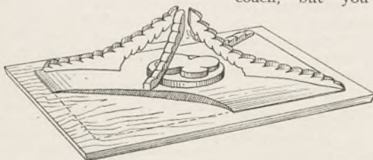
Fig. 5—The roof showing shaped overlay and ornamental portion ready to fix
