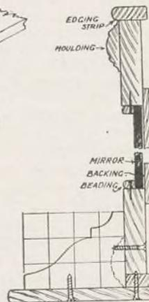
Fig. 5—A section showing various parts
