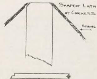
*Fig. 3—Side section showing V cut for string*
