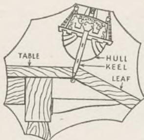
illustrated. A hinged support must be arranged beneath, as can be seen to hold the shelf tight at the correct height.—(L. H. Webb).
