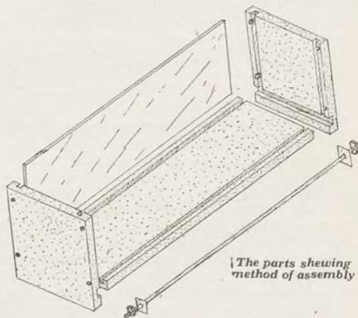
The formwork should be assembled and fastened down lightly to a solid wooden base, which will not warp appreciably when wet.
