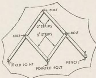
On the end of one of the 9 inch strips make a hole for a pencil to slip through and hold tightly. Now the pantograph is complete, but before using it make sure that all the joints are loose. To use it, place the pointed bolt round the design and an enlargement will be produced by the pencil. Of course this can be made with cardboard or meccano.—(F. Weller).
