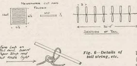
Fig. 6—Details of tail string, etc.
