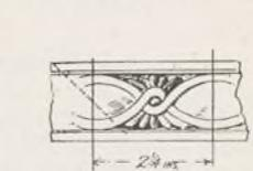
Fig. 4—Cut the moulding in sections as shown
