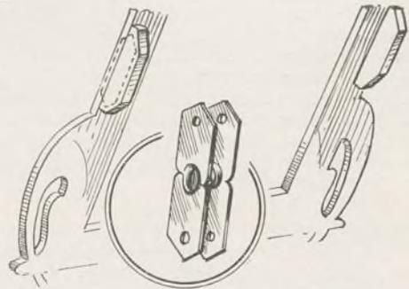
Fig. 3—The swivel parts and holders
