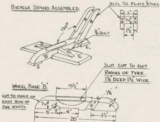
Oak was used in making the wheel-base, B, and wheel supports, A and A<sub>1</sub>, as much strength as possible being required here, while the remaining portions were of deal. Now as to working details: first take a piece of oak 20ins. by 2ins. by 2ins., at centre 10ins. from either end, cut a slot 9 $\frac{1}{2}$ ins. long, 1 $\frac{1}{8}$ ins. wide, and 1 $\frac{1}{2}$ ins. deep at centre, to suit radius of tyre.
