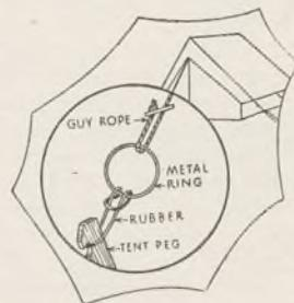
a guy rope which might result either in a broken guy or a ripped tent. First of all cut four rings 1/2 in. wide from an old motor inner tube and attach to each of these a small brass curtain ring. Then attach same to the guy as shown and you have only to slip the rubber over your peg (as previously the rope) and you have an excellent safety device.—(W. McFall).
