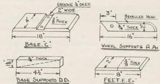
from a piece of deal 4 $\frac{1}{2}$ ins. by 1 $\frac{3}{8}$ ins. by  $\frac{3}{8}$ in. cut as indicated by dotted lines and held by 2 screws through base, C, and a small nail driven in from the top inside of slot of wheel-base, B, afterwards the head being filed smooth so as not to rub the tyre.
