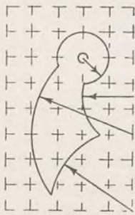
Fig. 3—Outline of adjusting piece, in \frac{3}{8} in. squares
