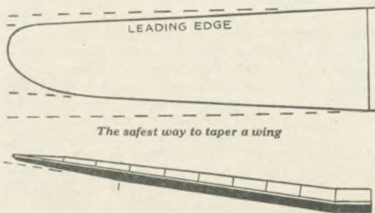
Showing "washout" (decreased incidence) at wing-tip
