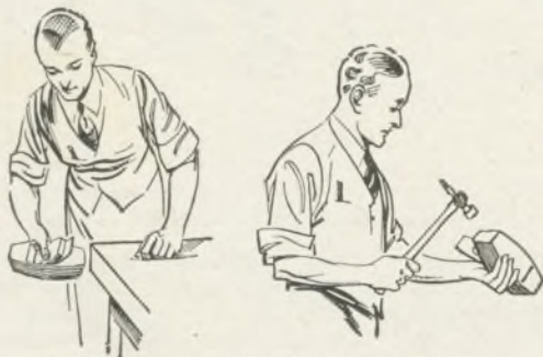
Two ways of releasing the plane iron
