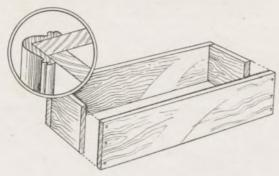
Fig. 1-Construction of a box with detail of corner
