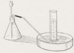
Fig. 4-The Preparation of Hydrogen
