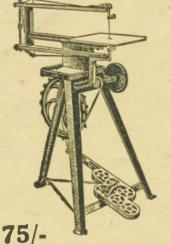
This is the "Triumph." It runs on ballbearings and is a heavily-built machine to stand up to long periods of service. It runs as "smooth as silk" and has a clearance of 19ins, behind the saw.
