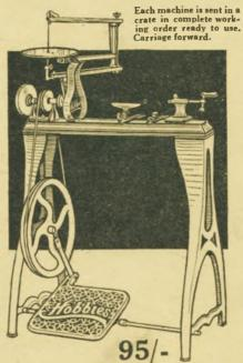
The "Companion" Lathe and Fretsaw is the ideal woodworker's machine. As can be seen it is a useful lathe 14ins. between centres with a fretsaw attachment mounted on top. This attachment can be taken off and put on again merely by unscrewing one nut. The large driving wheel has two grooves to give a change of speed.
