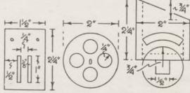
Fig. 3-Box end and rear wheel
