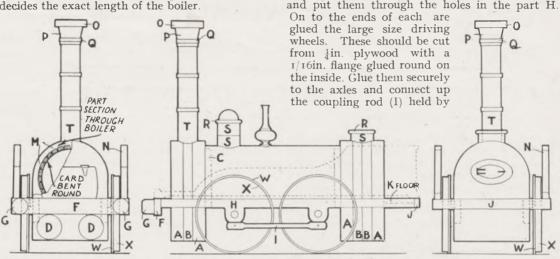
Fig. 3—Elevation of side and two ends of engine with lettered parts
