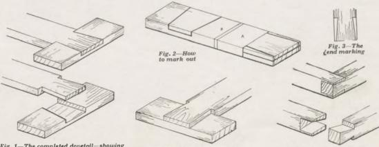
Fig. 1—The completed dovetail—showing the two portions
