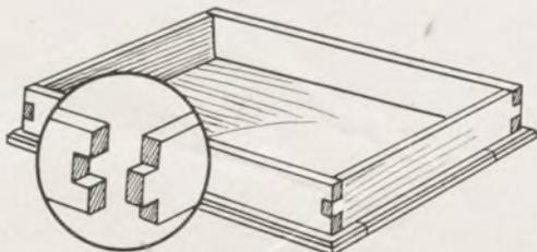
Fig. 2—The sides fitted, with detail of corner
