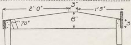
Fig. 3—A long section of the bed frame
