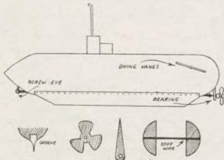
Section of keel    The 1 1/2 in. dia. propeller and shaft    Diving vanes
