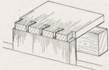
Fig. 7—Marking the cuts
