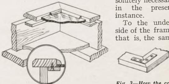
Fig. 3—How the corner plates are fitted
