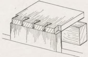
Fig. 7—Marking the cuts
