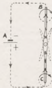
Fig. 2—Effect of current on Compass needle
