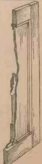
Fig. 7.—A broken away picture of the door, rails, overlays, etc.
