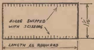
Fig. 5.—A piece of paper should be wrapped round the bobbin.
