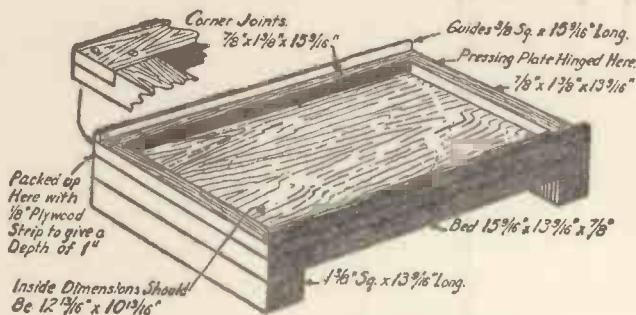
Fig. 1.—How to make the Press Bed.
