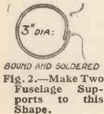
Fig. 2.—Make Two Fuselage Supports to this Shape.
