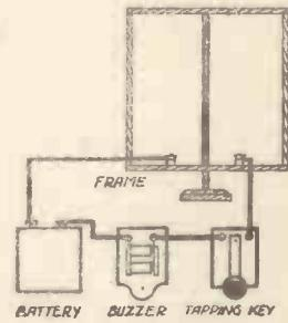
Fig. 6.—Substituting a Buzzer and Tapping Key for the Microphone.
