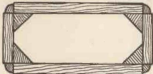
**Fig. 3.—A Section through the body of the Clock showing the Corner Blocking Pieces.**
