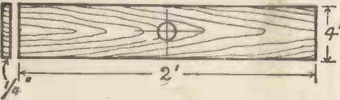
Fig. 2.—The Measurements of the Wood for the Frame Aerial.
