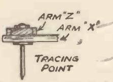
Fig. 4.—How the Tracing Point is made.
