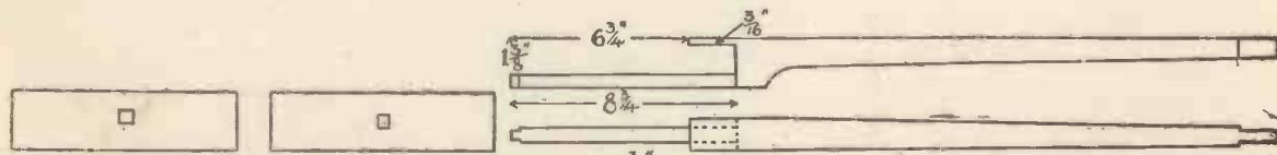
Fig. 2.—How the Holes are cut in the Ends of the Cigar-box.
