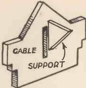
**Fig. 1.**—A Back View of the way the Gable is stiffened up.
