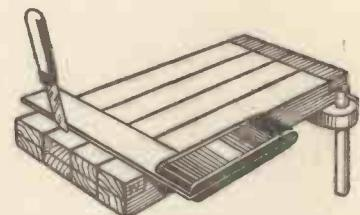
Fig. 4.—Setting out Rails for "Barefaced" Tenons.
