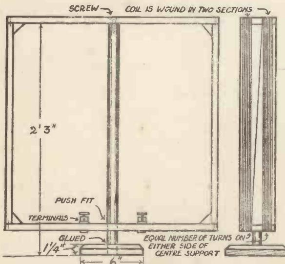
Fig. 4.—The whole Frame is supported by a length of Small-gauge Broom-handle.
