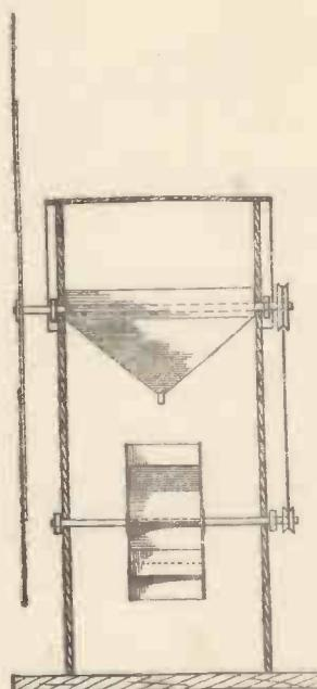
The Hopper and Sand-wheel Mechanism.
