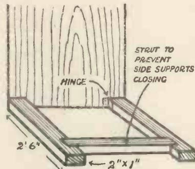
Fig. 2.—The Supports for the Front.
