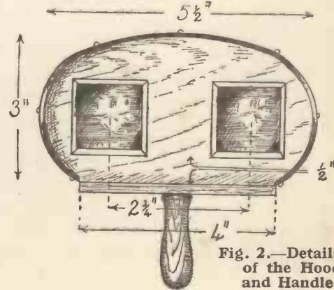
Fig. 2.—Details of the Hood and Handle.
