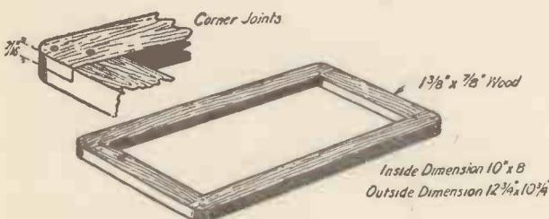
Fig. 3.—The Chase in which the Type is held or Set.
