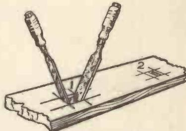
Fig. 8.—How to cut the Mortise.
