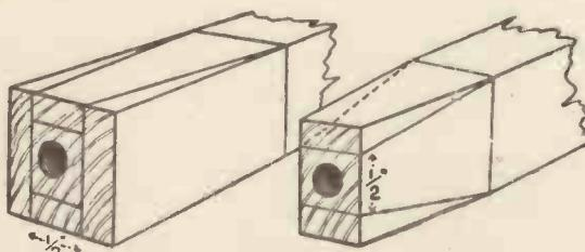
Figs. 3 and 4.—How to Shape the Front of the Barrel.
