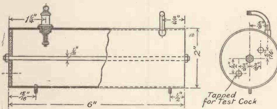
Fig. 3.—How the Boiler is made.
