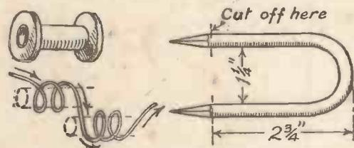
Figs. 2 and 3.—The Magnet and Coils.
