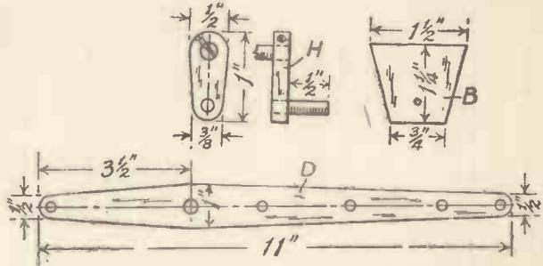
Fig. 3.—The Jib Winding Handle and Brackets for the Wheels.
