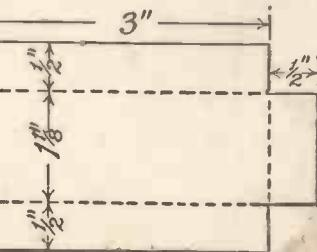
Fig. 10.—Tinplate Blank for forming Drip Tray of Lamp.
