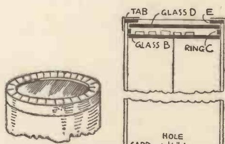
Fig. 4.—The Flat Ring of Card placed on one end of the Cylinder.
