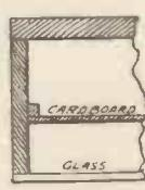
Fig. 2.—A Sectional View of the Box for holding the Sand.
