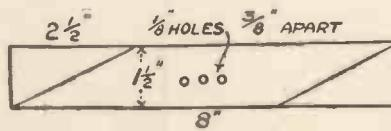
A piece of tin should be cut to the above dimensions and bent according to the flight required.
