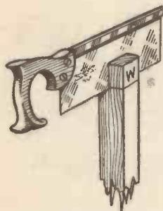
Fig. 5.—The piece marked "W" is cut away to make the Mortise and Tenon Joints.
