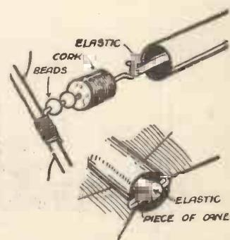
Fig. 9.—How to fix the Elastic in the Tube.
