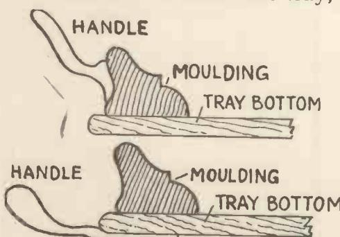
Fig. 3.—The manner of fixing the Handles is shown above. One is to the Moulding, and the other is under the Tray.
