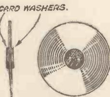
Fig. 5.—The Wheel with cardboard discs attached to strengthen it.
