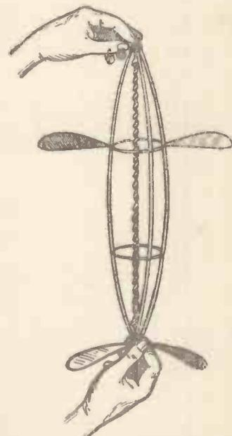
**Fig. 8.—How to launch the Model Helicopter.**
