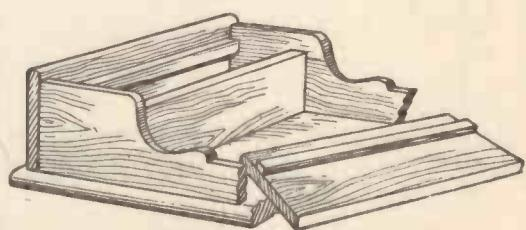
**Fig. 4. A detail of the Box fitted into the end of the Tray. The lid is shown away.**
