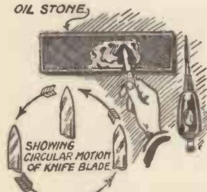
Diagram showing how to sharpen a pocket-knife blade on an oil-stone.
