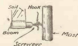
Fig. 3.—How the Boom is secured.
