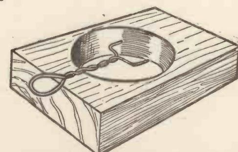
Fig. 4.—The mould for the lead weight.
