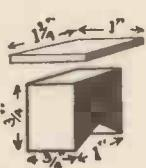
**Fig. 7.—How to make the Stacks for the Chimneys.**
