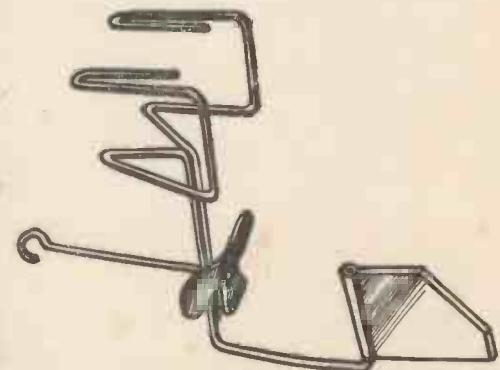
This diagram shows how to make the clip for the Rudder and the Propeller.
