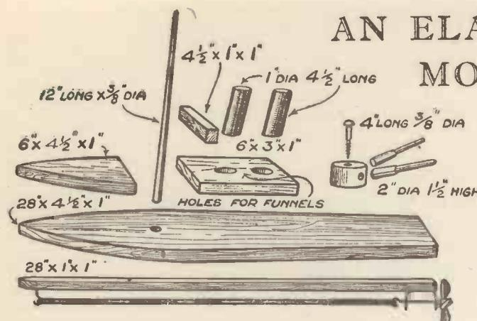
**Fig. 2.—The Component Parts of the Battleship.**
