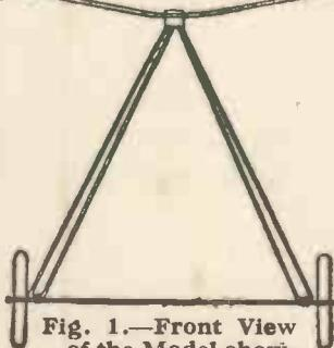
Fig. 1.—Front View of the Model showing the Dihedral Angle.
