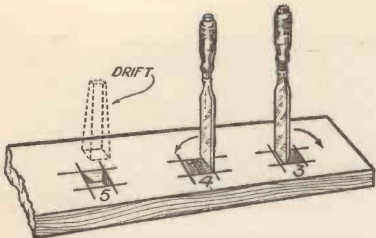
Fig. 10.—Showing the "Drift" which is driven through to remove the Waste Pieces of Wood adhering to the Sides.
