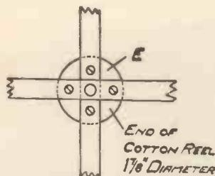
**Fig. 4.**—A Cotton Reel is used, as shown here, to form the Hub.
