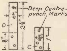
Fig. 5.—The Bearing Supports.
