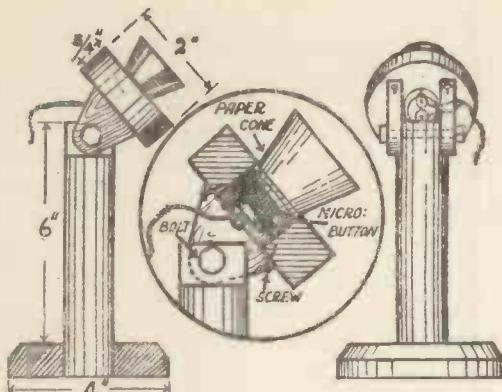
Fig. 5.—The Stand for the Microphone.
