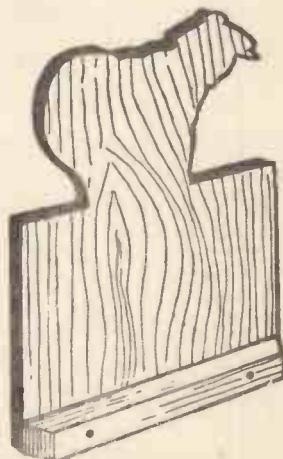
Here the Base is merely a strip of wood glued and nailed along the back.
