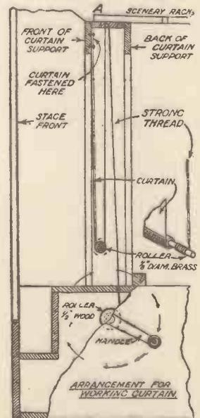
This Diagram explains how to work the Drop Curtain.
