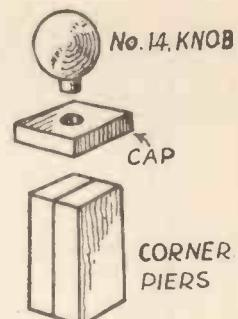
**Fig. 4.**—The Corner Posts of the Porch are made like this.
