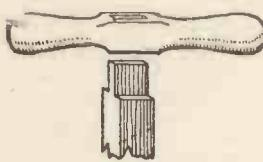
Fig. 4.—How to fix the Handle.
