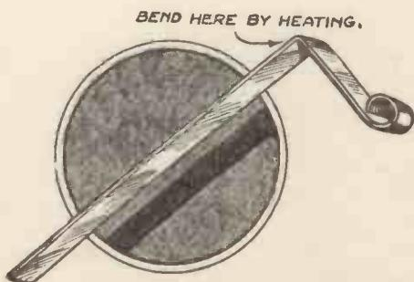
Fig. 7.—The Firing Spring.
