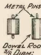
Fig. 7.—The Spindle Supports.
