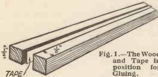
Fig. 1.—The Wood and Tape in position for Gluing.
