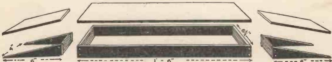
Fig. 3.—The method of making the Three Portions of the Platform.
