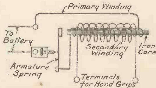
Fig. 4.—The Coil should be Tested by connecting up to a Dry Cell.
