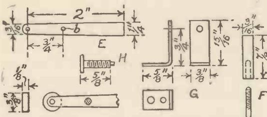
Fig. 3.—Details of the Contact Screw and Bracket.
