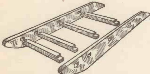
Fig. 11.—The Sides ready to be fixed together.
