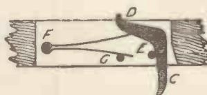
Fig. 4.—The Trigger for releasing the Bolt.
