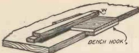
Fig. 6.—The Rail held on Bench Hook to Saw Tenon Shoulder.
