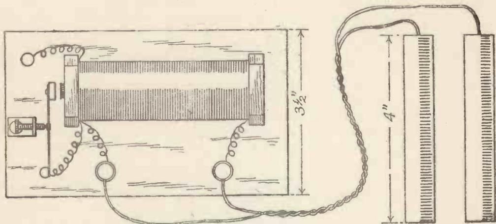
Fig. 1.—Plan View of the Shocking Coil.
