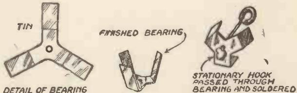
Fig. 1.—Details of the End Bearings.
