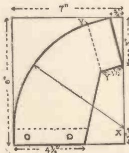
Fig. 3.—The details of the Neck Piece.
