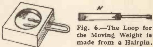
Fig. 6.—The Loop for the Moving Weight is made from a Hairpin.
