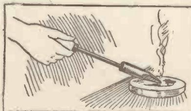
How to tin the Soldering Iron.
