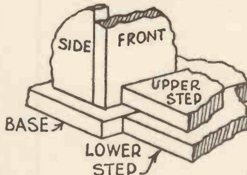
**Fig. 3.**—A Detail of the Front Corner of the House.
