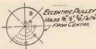
Fig. 6.—The Eccentric Pulley.
