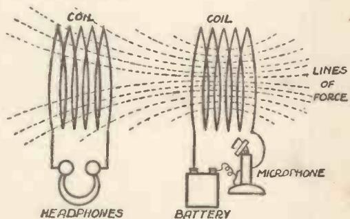
Fig. 1.—The Principle on which the Telephone works.
