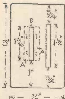
**Fig. 5.—The Top of the Box, showing the Position of the Dog and Money Slot.**
