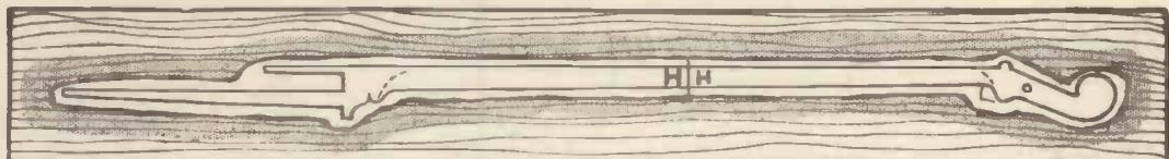
Fig. 1.—The Pattern of the two parts of the Neck are pasted on the wood like this, to make one complete Length.
