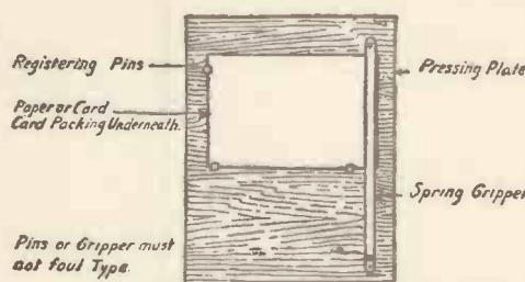
Fig. 5.—The Method of Registering the Position of the Type.
