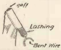
Fig. 2.—The "Gaff" is secured as shown.
