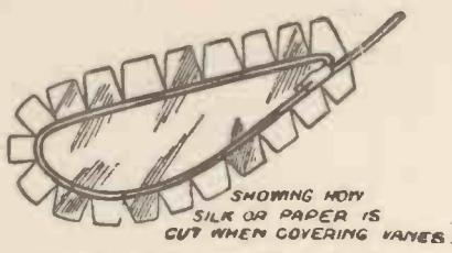
**Fig. 5.—How to cover the Wire Propeller.**
