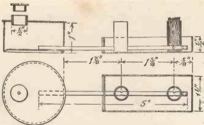
**Fig. 9.—Sectional Elevation and Plan of Spirit Lamp.**
