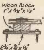
Fig. 3.—The Block for Clamping the Pantograph to the Drawing Board.
