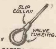
**Fig. 7.—How to form the Hook on the Propeller Shaft.**
