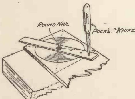
Fig. 4.—Cutting Discs from Plywood.
