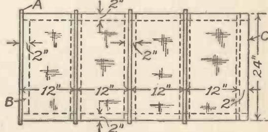
How to mount the Strips of Wood on to the Coloured Paper.
