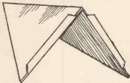
**Fig. 2.**—The False Roof to the Gable.
