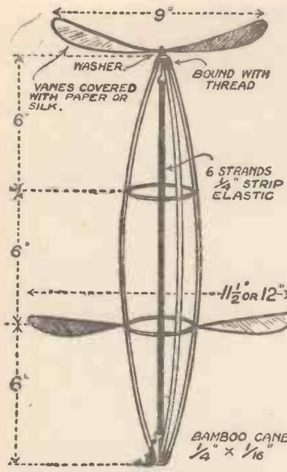
Fig. 3.—The Completed Model Helicopter.
