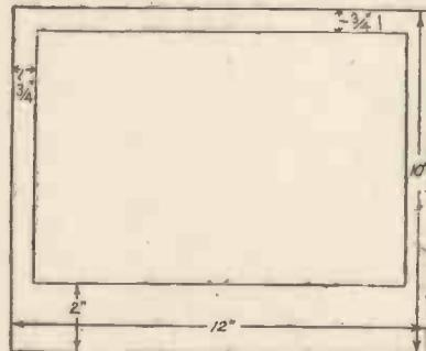
The Wood Frame on which the mounted Stage Front is Fixed.
