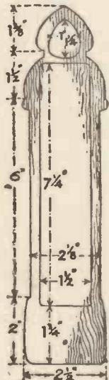
**Fig. 1.**—The measurements of the Pencil-Box.
