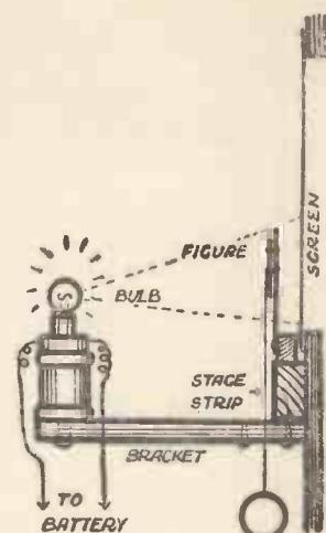
Fig. 5.—The Lighting Arrangement.
