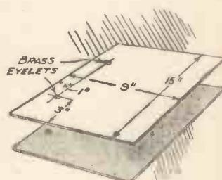
Fig. 7.—How to make the Cover.
