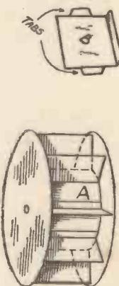
Assemble the Sand-wheel in the manner shown here, (A) the Core, and (B) one of the Blades.
