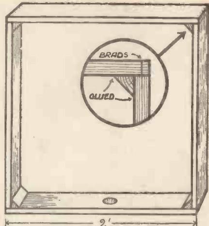
Fig. 3.—How the Frame Aerial is assembled. Inset gives details of the Corner Joints.
