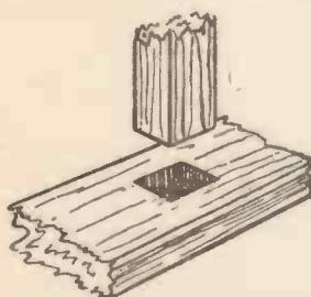
Fig. 1.—The Base with hole cut to take the upright.
