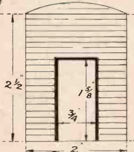
Fig. 2—End view with doorway
