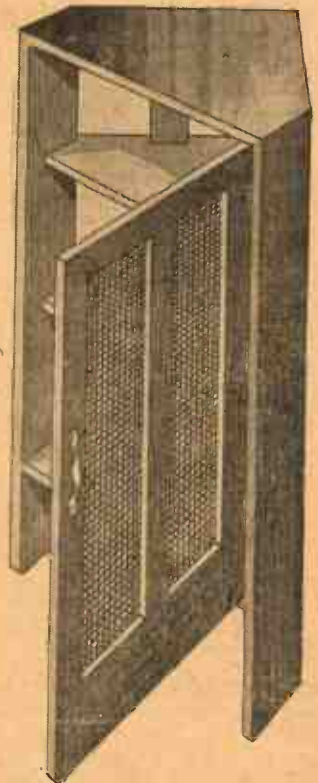
This practical piece of work stands just 2ft. 6in. high and 12 \frac{1}{2} in. by 14 \frac{1}{2} in. wide.
