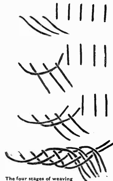
The four stages of weaving
