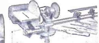
Showing Sanding attachment replacing Saw. (left) Super Swivel Platform positioned for turning at any angle (front, rear or end).
