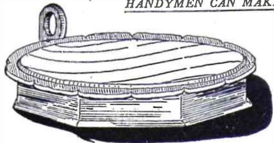
THE common plate, with its raised rim, is not the ideal article on which to cut a cake, especially a soft one, inclined to crumble. The cake-board illustrated, provides a flat foundation for the cake to rest upon, and renders the job of cutting it into slices an easy one. As the board can be rotated by the fingers, it is not necessary to keep turning the cake itself to find a fresh portion to cut, it comes to you. Nicely finished, the article would make an attractive table feature as well.
