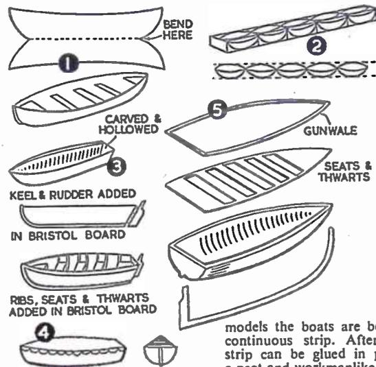
of small open boats are required. It is only recommended, where the model-maker is doubtful about being able to carve and hollow them from the solid, and is included only to enable the beginner to make a model of a small open boat that will give an in-scale appearance.
