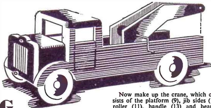
Now make up the crane, which consists of the platform (9), jib sides (10), roller (11), handle (13) and bearing piece (14). The pieces 13 and 14 are
