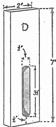
Fig. 4—The sliding column
