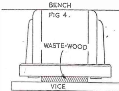
Instructions are given for making a stand to take a photograph up to 4ins. square. The height may be increased in proportion to the width if a larger photograph is to be accommodated. A mild-grained hardwood should be used. For the base you will need a piece of wood 7½ins. by 2ins. by 1in. This is trued up to finish 1½ins. wide and ½in. thick. The marking out is shown in Fig. 1. It is the distance between the
