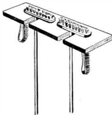
board 6ins. wide and 1in. thick to fit in the corner. This can be fitted and held by brackets at a convenient height. The slots are cut to whatever depth is needed as long as enough is left to keep the board in shape. You can get four
