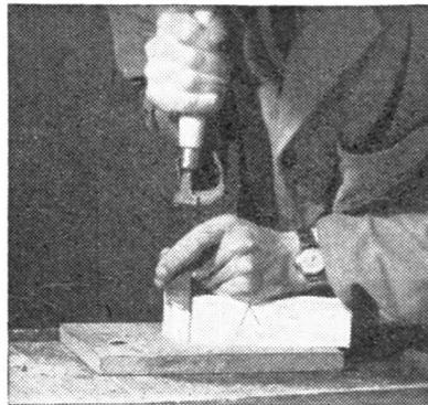
slice you can manage. The chiselling board must be kept free of chips, so that there is no space between the board and the wood. (K.B.)
