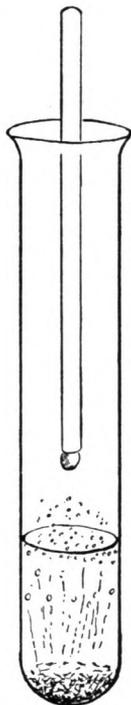
Carefully lower a glass rod carrying a drop of lime water into the test tube
