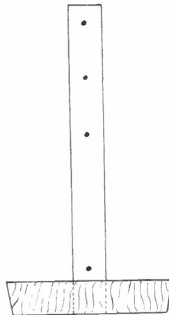
to drain away as soon as washed out of the prints. Other holes are drilled higher up the tube to hasten the drainage as the water rises in the sink. (S.H.L.)
