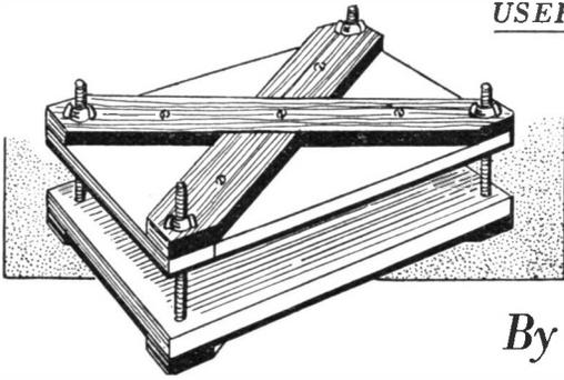
FOR many articles of woodwork a press is very necessary. Other crafts also, besides woodwork, need a press at times, and the simple but efficient type illustrated is, therefore, well worth making. The construction of a cheap design of cramp is also included in this article, just the thing for doors and frames generally.
