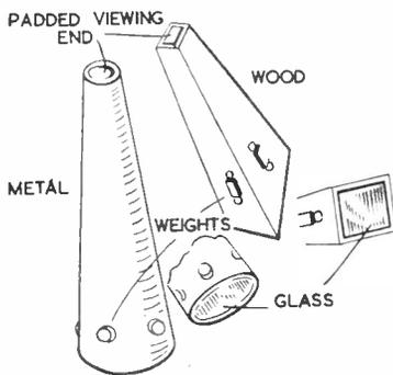
bottom to counteract the buoyancy of the air which is contained in the funnel, and they also help to submerge the big end. Paint the inside of the funnel black to prevent the light from being reflected on the bright surface of the
