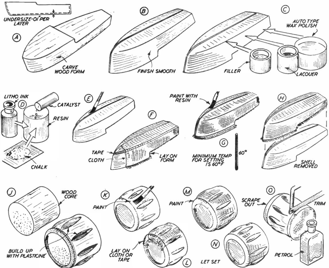
with a strength comparable to that of mild steel. It is a thermoset plastic, which means that it will not soften or distort when heated. In other words, once 'set', it is set for good. It can only be worked by treating like a metal, such as filing, drilling, sawing, etc.
