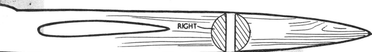
CUT ONE OF EACH 1/4IN. SHAPE TO SECTIONS ONE LEFT - ONE RIGHT
