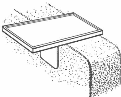
ALL too often, a well-deserved rest is interrupted because a cup of tea refuses to balance on the arm of the chair. But with a little effort, a small but serviceable tray can be constructed, which will fit on the chair as shown in the illustration. It can be adjusted to suit most armchairs, and will fold flat when not in use.
