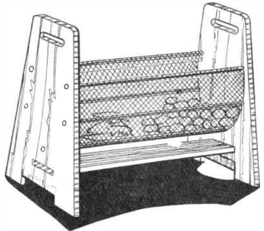
shown in Fig. 3. Tap the floor and dowels in position a little at a time. Do not try to push the first one right home or you will not get the others in position. Remember that a little glue should be added to each joint.
