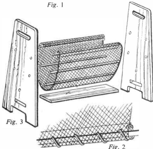
The advantages of this type of rack over that made solely of wood are obvious. The vegetables are seen clearly through the wire mesh and you can tell at a glance when they need replenishing. This is a good point as far as the shopkeeper is concerned, because his customers can see the produce without handling.
