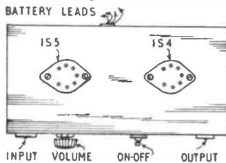
Fig. 2—Top layout and valve positions
