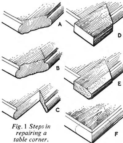
Fig. 1 Steps in repairing a table corner.
