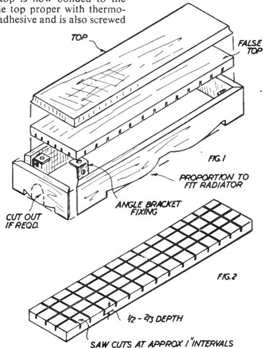
in place, from the underside. Make sure that you choose a screw length less than the total thickness of the two top pieces. Check also that the jointing is done over a true surface, so that the laminated top comes out perfectly flat. If screws are used as well as glue, there is no need to clamp these two pieces
