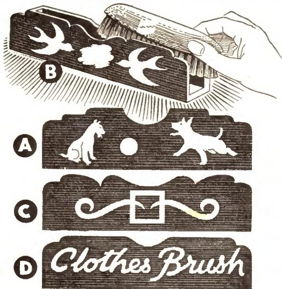
wood, and the bases (2) and back (1) and end piece (3) from 1/4 in. wood.
