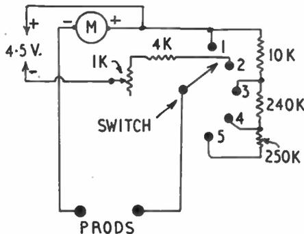
Fig. 3—Circuit for 5 range meter
