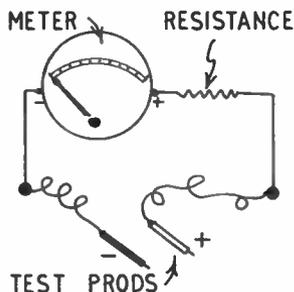
Fig. 1—Circuit for measuring volts
