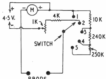
Fig. 3—Circuit for 5 range meter
