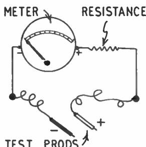
Fig. 1—Circuit for measuring volts
