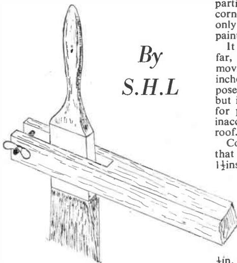
**T**HERE are times when one wishes the paint brush had a longer handle or could be made to extend a little further to avoid moving the ladder so many times. This applies
