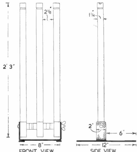
in the side and front views in Fig. 1. Notice that the base is made from  $\frac{1}{4}$  in. mild steel 2ins. wide. It can be riveted or welded together as shown in Fig. 2. The inside measurement of the 'U'-shaped piece is exactly 8ins. and allowance should be made when bending or the measurement will be scant.
