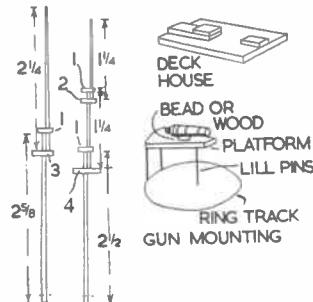
wood and treated with shellac instead of painted. Make the mast assemblies and bind and glue the spars in place. In fixing gaffs and booms on small models, a short length of lill pin inserted in the end of the spar and driven into the mast when gluing in position makes a very strong job of the joint.
