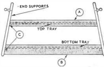
drawing parallel pencil lines  $\frac{1}{4}$ in. apart. The ledges are cut from  $\frac{1}{4}$ in. square hardwood. Note that they fall short of the edge of the main supports by  $\frac{1}{4}$ in. at each side — i.e., the thickness of the side pieces (A and B). Plane one face of each ledge strip at an angle to allow for the eventual lean of the end supports. Glue them in place between the pencil lines and reinforce each by driving three woodscrews through the ledge into the supports.
