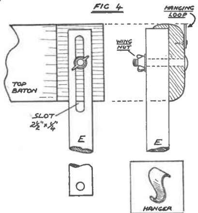
the palm resting on one of the verticals, and an upward pull is given, the final turn to the wing nut at this side being given when a good tight stretch has been secured. Having stretched one side, proceed to stretch the other.
