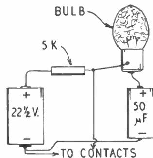
Fig. 3—Capacitor firing
