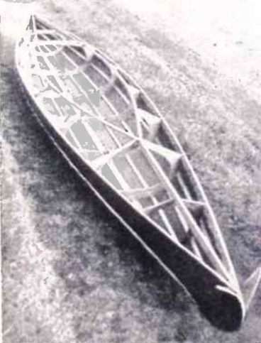
The framework varnished and the hull canvas fitted, ready for fixing the keel and bilge keels, followed by the deck.
