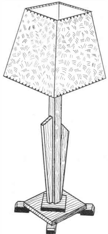
A start is made by fixing the two base boards together, the jointing surfaces being glued and four small screws driven in from underneath.
