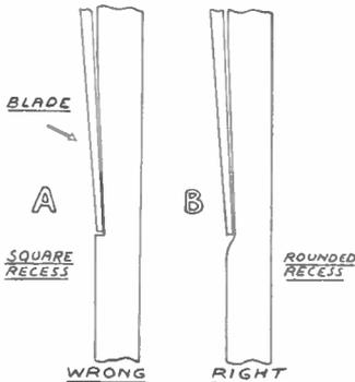
Wrong and right way of recessing the rail at the blade tip.
