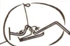
SHOWING HOW CONTROL ARM OF MUSICAL MOVEMENT IS BENT AND SPRING RELEASED
