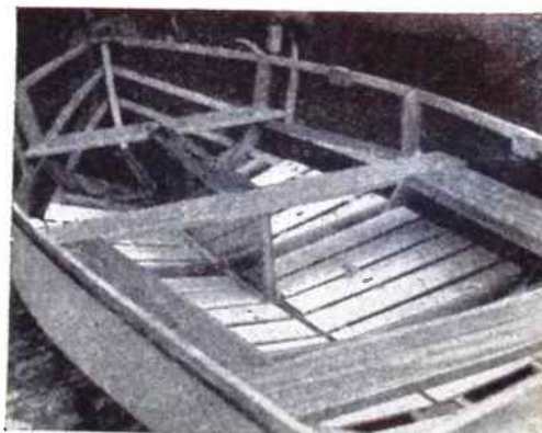
The hull completed for sailing, with the centreboard fitted in its case and side benches between the thwarts
