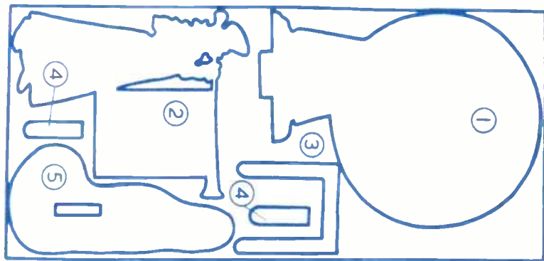
Fig. 1—Showing how the various parts are laid out on the panel of wood
