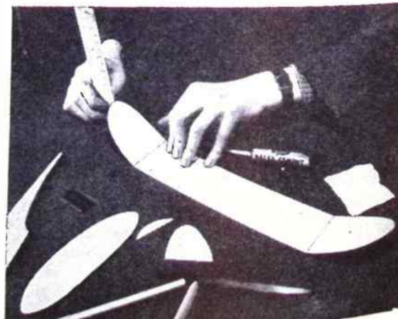
Checking dihedral on wing tips
