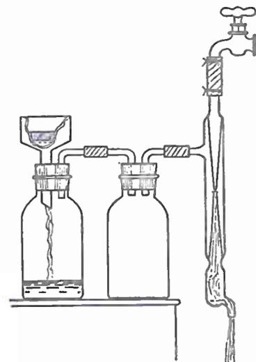
Fig. 2—Filtering hydroferrocyanic acid under reduced pressure
