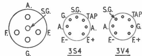
Fig. 2—Valve connections
