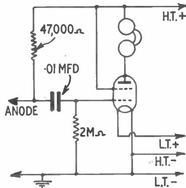
Fig. 3—Resistance-capacity coupling
