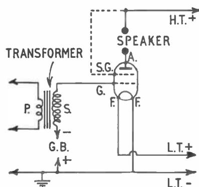
Fig. 1—Transformer coupling
