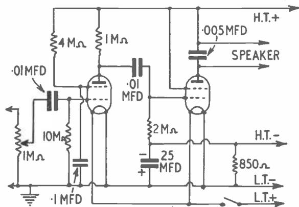
Fig. 5—A 2-valve amplifier
