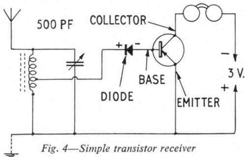
Fig. 4—Simple transistor receiver
