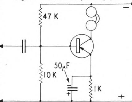
Fig. 8—Amplifier with emitter bias
