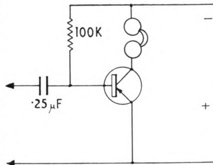
Fig. 7—Condenser coupled amplifier
