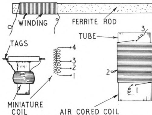
Fig. 6—Some coils for transistor circuits
