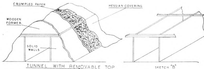
dowel and glue them into the stringers, say one at each end, and about 1 in. in from the end, and one in the middle. You will readily see that these dowels and holes are to hold the top on without it moving.
