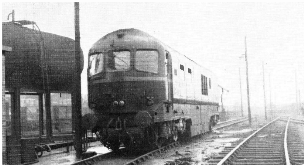
The B.R. Western Region gas turbine locomotive No. 18000 at Old Oak Common
